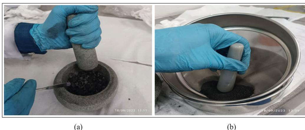
Figure 2. (a) The process of crushing PAC material using a mortar and pestle after carbonization, and (b) the process of sieving the PAC Powder using a < 20 micron sieve
